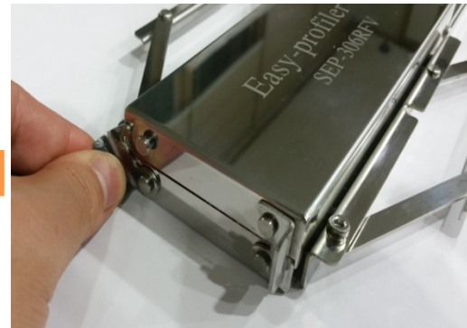
Ass'y hanger 2 point against Sensor .
