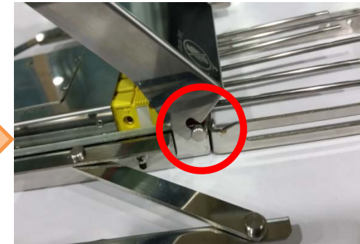
Assembly ( Upper case +Lower Case of sensor hanger )
